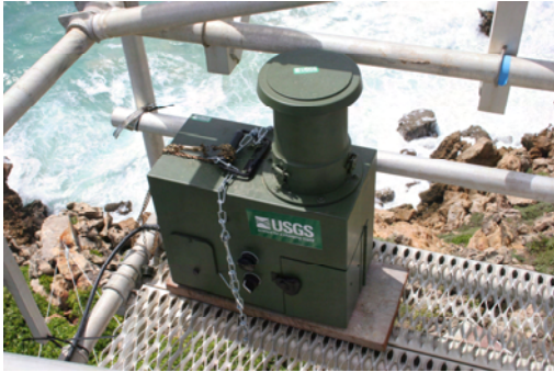
Photo courtesy, Dr. Christina Kellogg, USGS This Kellogg Sampler unit in Barbados captures dust samples and any accompanying bacteria blown across the Atlantic Ocean from the Sahara desert.
